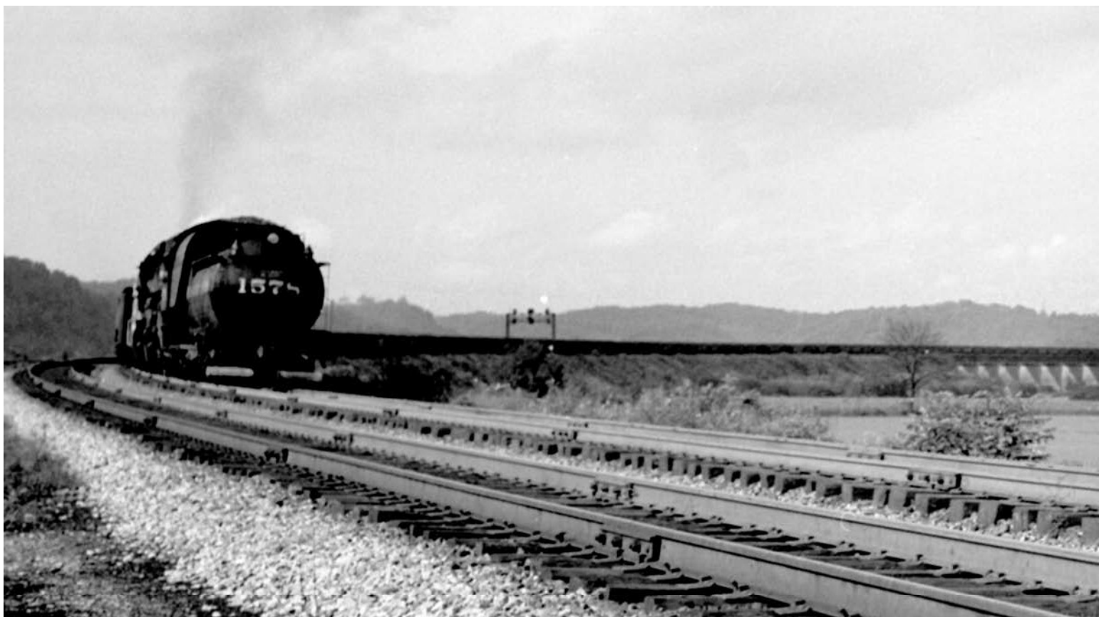
H-7 2-8-8-2 No. 1578 shoves a westbound coal train up the steep approach to Limeville bridge in September 1950. Note the smoke from the lead engine in the distance beyond the bridge. After the train's rear had reached the bridge the pusher would return to its pocket near NJ Cabin at Limeville Junction. (Gene Huddleston Photo, C&OHS Collection, COHS 1446)
